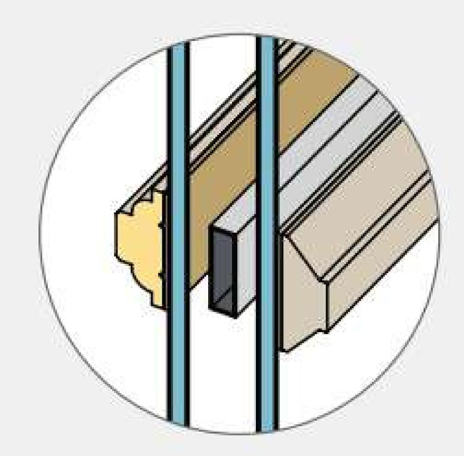
Powerful Design in a Look You Love Simulated Divided Lite (SDL) grilles blend cutting-edge modern efficiency with timeless aesthetics. These grilles replicate the appearance of classic single-pane windows, but pack powerful insulation in the form of exterior and interior grille bars, with or without an aluminum spacer bar for maximum efficiency.
